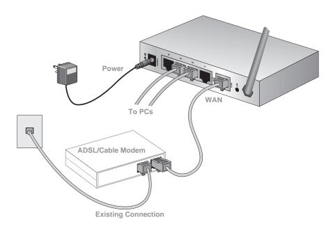
Figure 4 Installation Diagram
